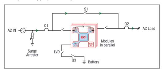
Flexa - Subrack System - By-Pass Mode Operation
