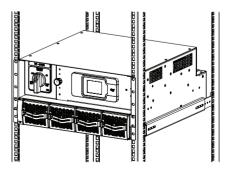
**Step 4.** Verify the correct slot for each module and place the module.
