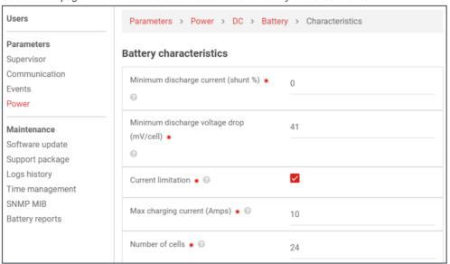
Enter the battery parameters such as charging voltage and current, number of string and its capacity, number of cells, and so on.
