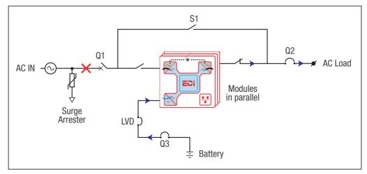
Flexa - Subrack System - Battery Mode Operation
